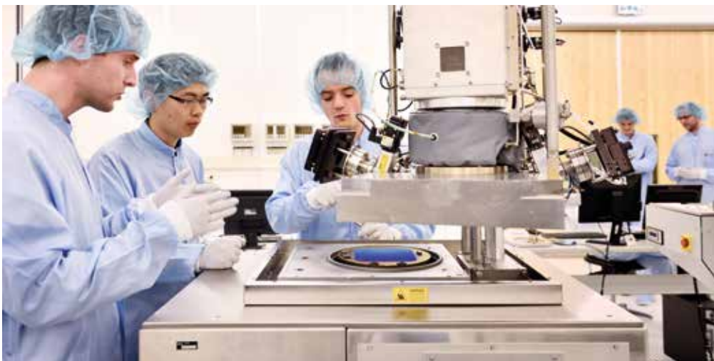
Zonnecel- en atoomlaagdepositiereactor in cleanroom, Tu/e.
